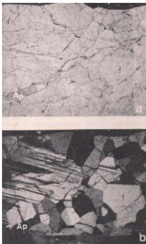
Figure 12: Thin section photomicrograph of magnesian anorthosite clast in 14321,1273 (figure 1 from Lindstrom et al. 1984). Scale is 2.3 mm across.
