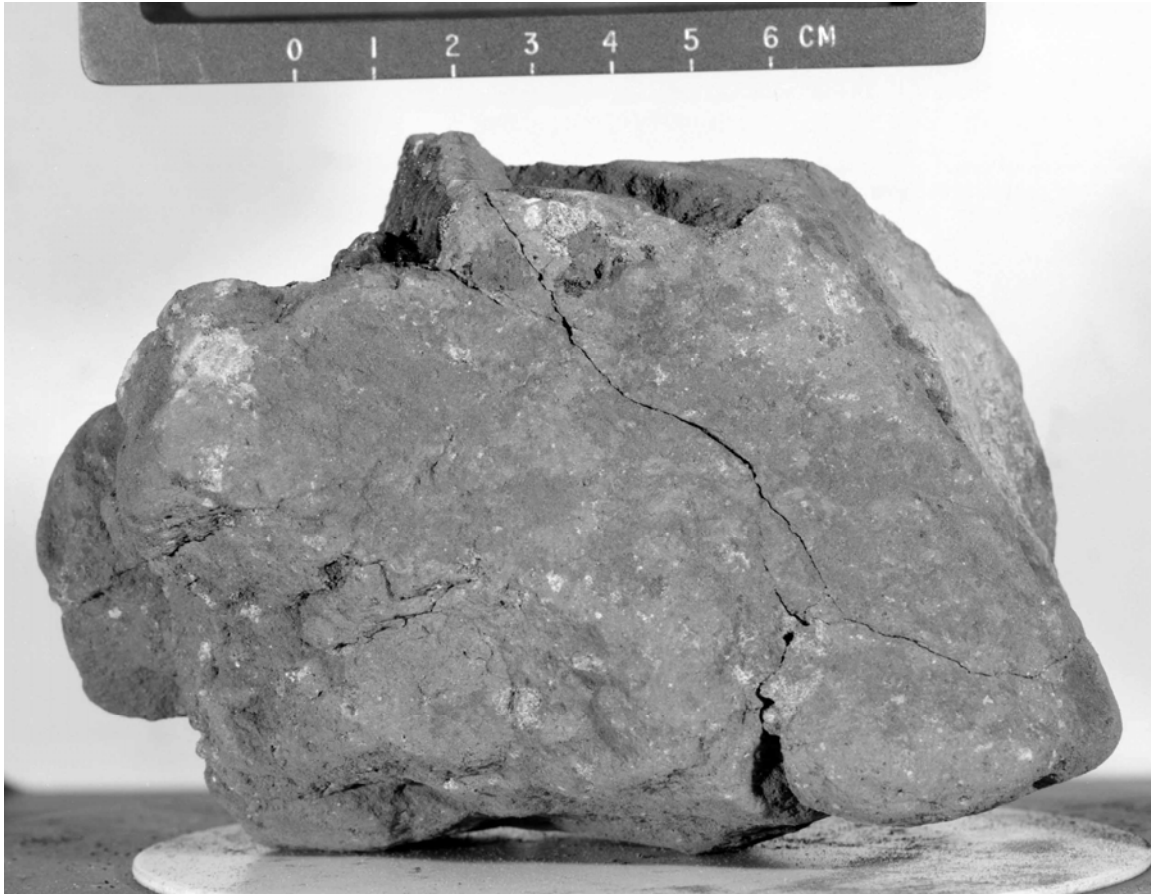
Figure 1. Macroscopic views of original sample showing fractures, glass patch, basaltic clasts, and zap pits. S-71-45129 and S-71-45163
