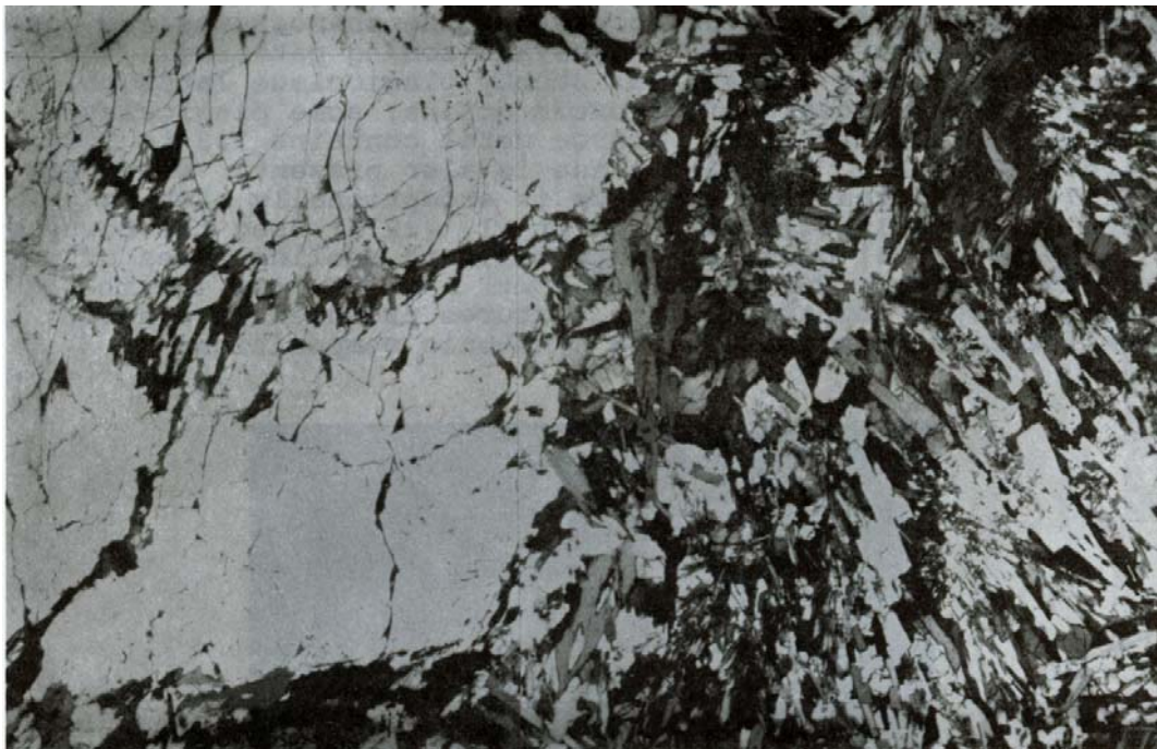
Figure 2. Photomicrograph of 15118,6, showing large irregular phenocryst (left) and contrasting groundmass (right). Crossed polarizers. Width about 2.5 mm.
