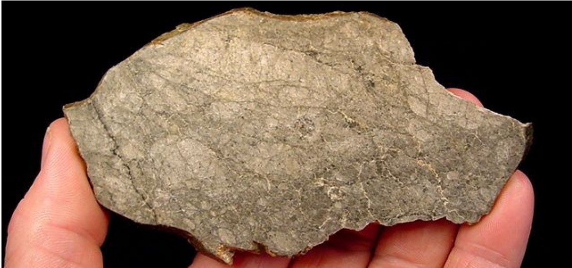
Figure 2: slab cut of NWA 3163 illustrating the feldspathic nature of the sample, as well as the thin veins (photo from R. Korotev).
